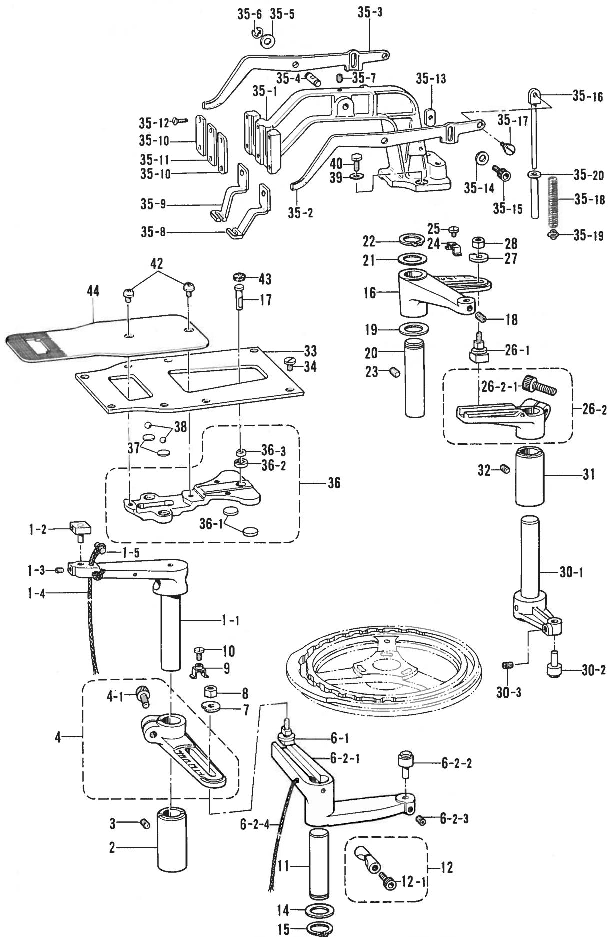
F. 送り関係/Feed mechanism/Transportvorrichtung/
