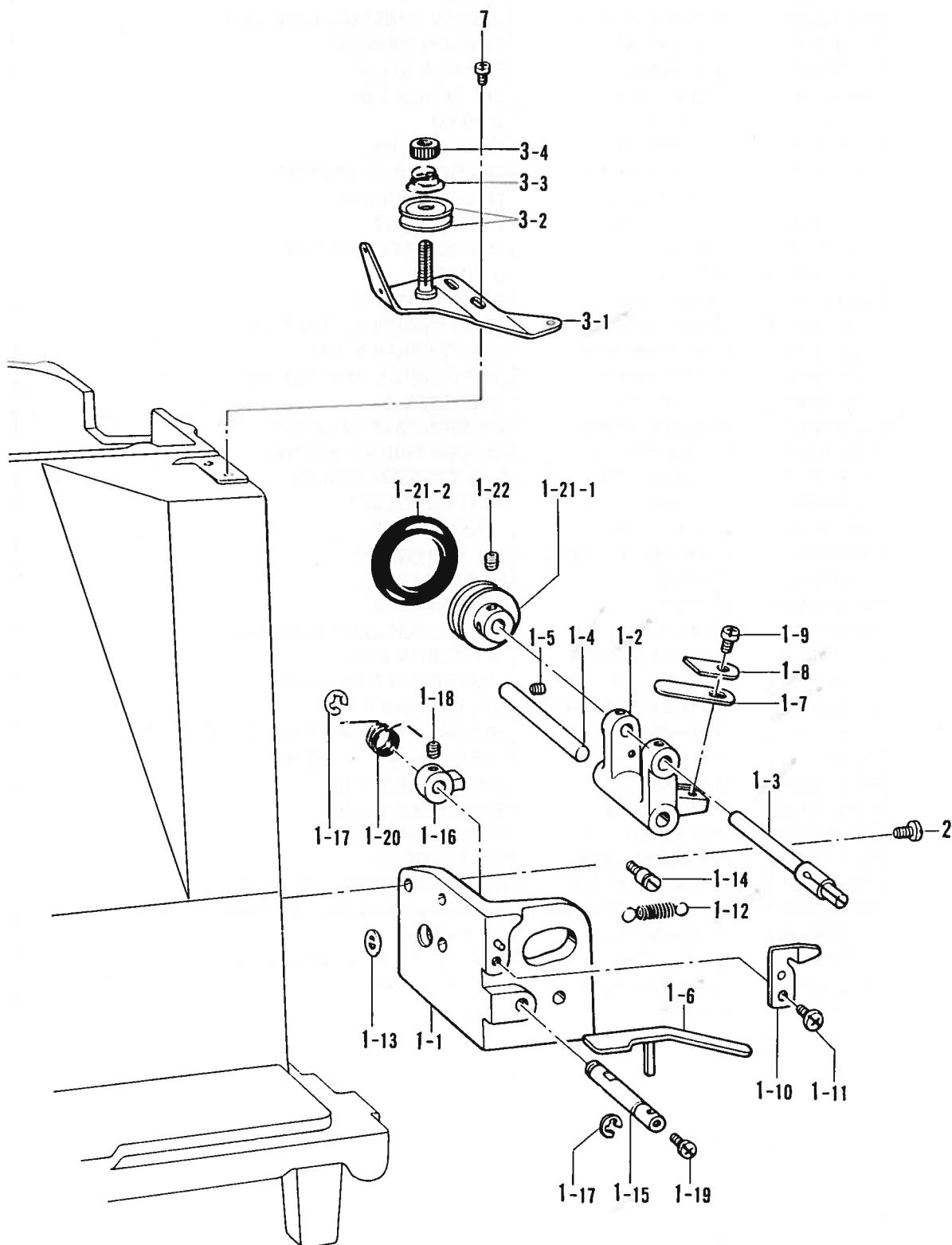
N. 糸巻キ関係/Bobbin winder mechanism/Spuler/
