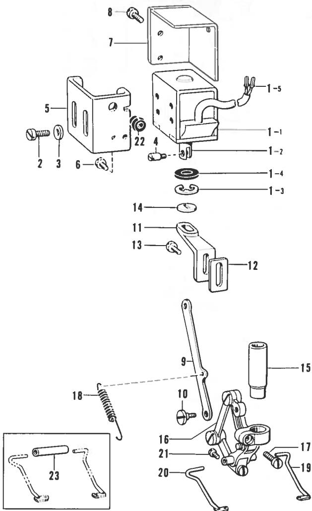
P. Quick reverse switch mechanism [-400A..-700A..-900A]
