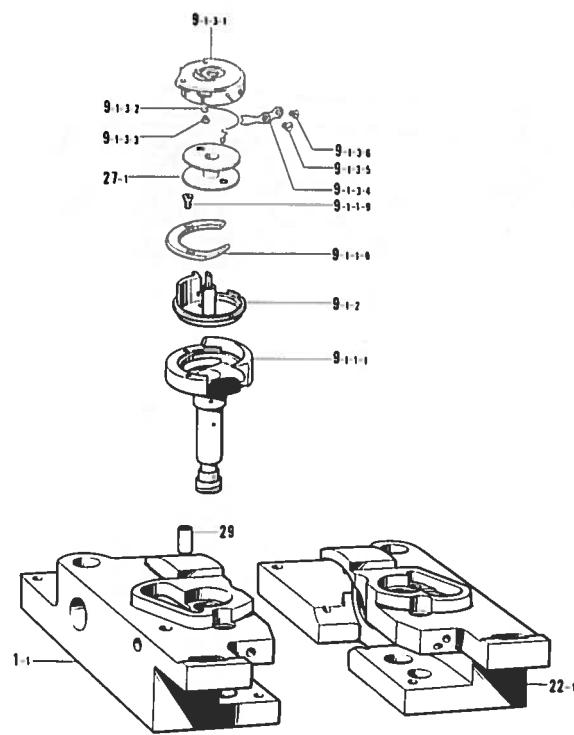
**K. Rotary hook mechanism (3)[-400A--700A--900A]**
