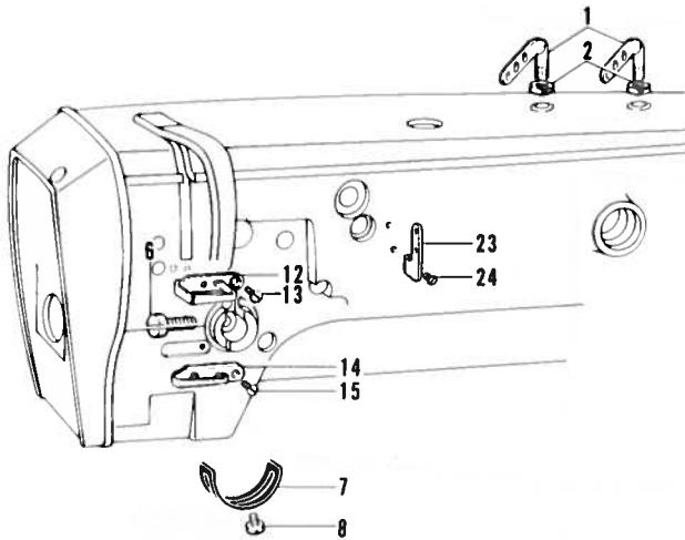
**B. Threading mechanism (2)(Standard)**
