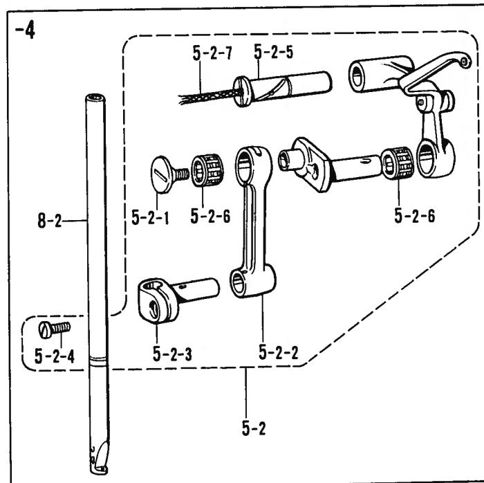
B. 針棒関係 /Needle bar mechanism/Nadelstangenvorrichtung/
